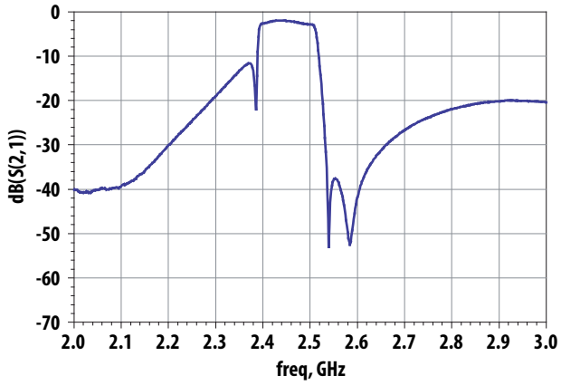
Figure 1. TX Path 2 – 3 GHz Frequency Response
